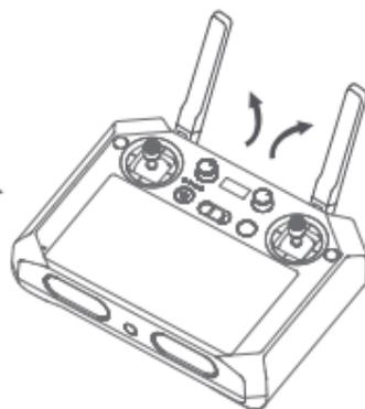
Unfold the antenna
